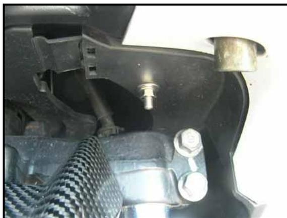
5. Replace the speedometer cable with an electronic type wire.
