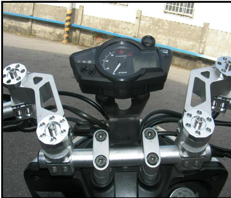
Picture to the left, shows the gauge installed on the original mounting bracket. The gauge is secured to this bracket by two bolts. Make sure the rubber anti-vibration boots supplied with the kit are installed. The PGO gauge is waterproof, so it is safe to wash the gauge and ride in the rain. Install the rubber boot for the wire harness correctly to protect the plug/wire harness from moisture/dirt. Cover exposed wires with elastic non-conductive tape.
